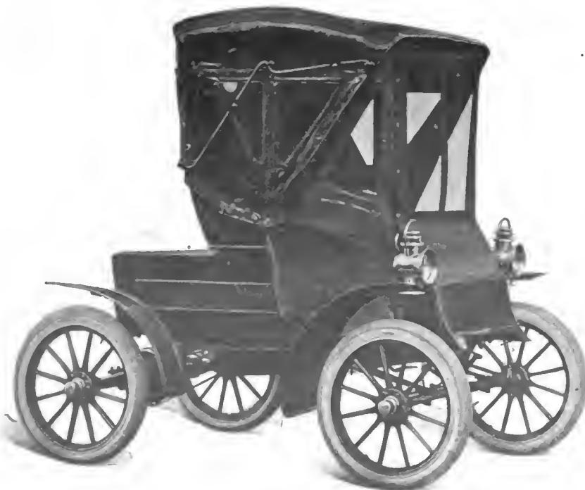
NORTHERN 7-HORSEPOWER RUNABOUT FITTED WITH FOLDING TOP AND WIND SHIELDS.
